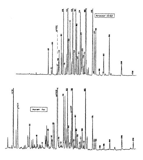
Figure 1. Temperature programmed capillary column ECD chromatogram of a standard (Aroclor 1260) and a sample of human fat. Chromatographic conditions as follow: carrier gas Argon/Methane (95/5) 100KPa; detector 300°C; injector 280°C; temperature programme, isothermal phases at 100°C (2 min) and 280°C (10 min), with intermediate temperature increase rate of 3°C/min.
